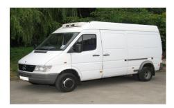
This diesel Mercedes Sprinter van has been fitted with refrigeration equipment, meaning that the value of this vehicle to the owner remains high. The Gross Vehicle Weight of this van is 3,300kg and the unladen weight is 1,705kg. This means the Low Emission Zone applies to this vehicle from 3 January 2012.
